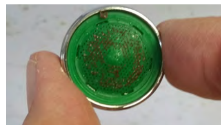
Aerator with sediment
